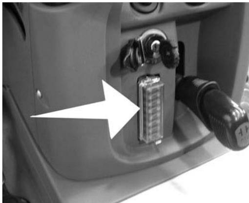
The electrical system is protected by fuses which are grouped in a plastic fusebox located under the bonnet close to the dashboard.
